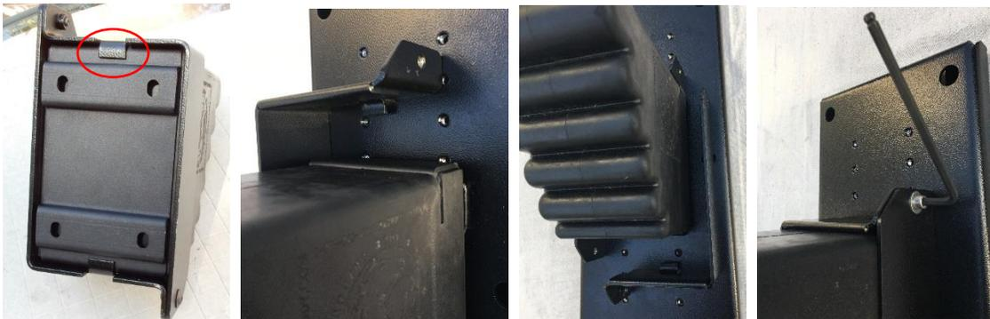
Finally, fasten them together with the flat washers and ¼-20 x ½” socket head cap screws using the 3/16” Allen wrench as shown above.
